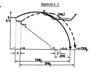
Assuming that the order was received at a time au and reduced stocks to S-1, the repairable part j returns after  $TPR_j$ . A logistic failure occurs at point  $\tau+t$ , when demand number S+1 arrives. If the probability of this occurring in interval  $(\tau+t,\tau+t+dt)$  is
